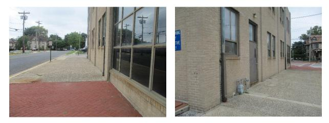
Downspout planter boxes on the east side and stormwater planters on the west side of the building can capture rainwater from the roof to be used to irrigate landscaping as well as reduce stormwater runoff into the sewers. A preliminary soil assessment suggests that the soils have suitable drainage characteristics for green infrastructure.
