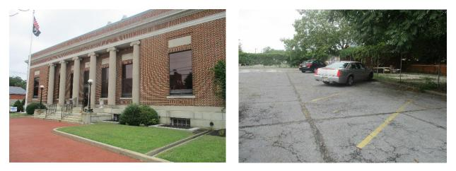
By replacing parking spaces with pervious pavement, the parking lot may capture rainfall and allow it to be filtered and infiltrated into the ground. A preliminary soil assessment suggests that the soils have suitable drainage characteristics for green infrastructure.
